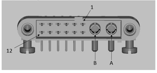
Connector Type: Manufacturer: Manufacturer Part No.: Mating Cycles: *Mates With:*  CMM Micro Connector, 2x Male HP contacts + 12x Male LF contacts Nicomatic (<u>https://www.nicomatic.com/family/3</u>) 221∨12F23-0200-3400CMM ≥500 222S12M16C-0200-4320 (Nicomatic) M80-4C11205F1-02-325-00-000 (Harwin) 14143-25 (Nicomatic)
